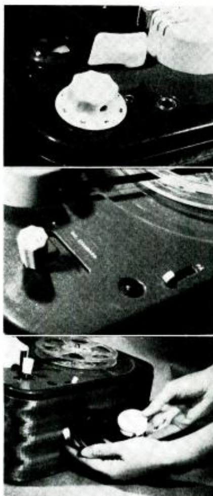
Top: the left side of the top showing the magic eye, volume control and mode selection lever. Center: the function selector in play or record position and the on-off switch. Lower: the mike and cords fits in a side well.
