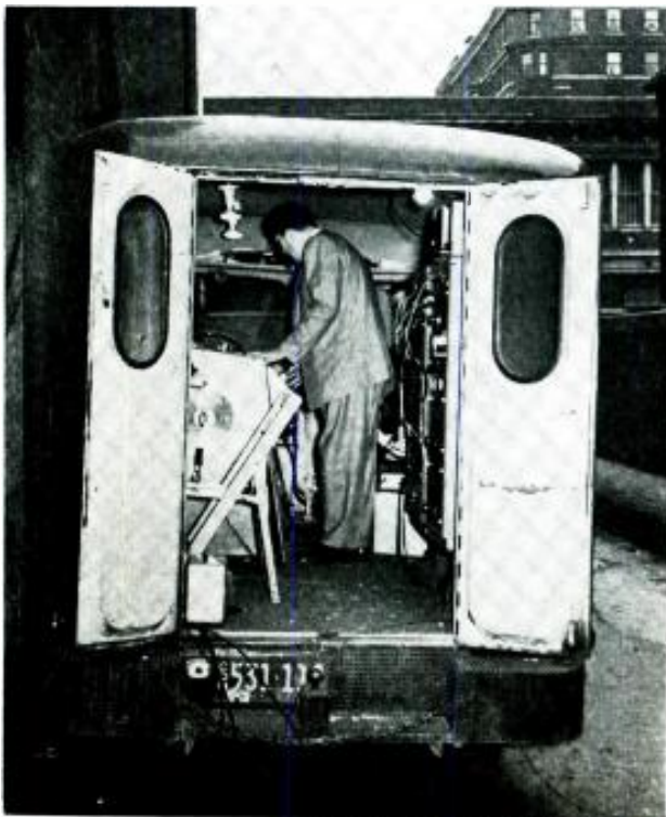
Left: the portable sound recording truck of Fine Sound, Inc. is loaded with equipment. Here it is parked in an alley behind Detroit's old Orchestra Hall ready to record the music from inside. Above: recording engineer Aaron Nathanson checks one of the Fairchilds inside the truck. The monitor speaker is above the recorder.
