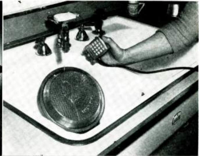
You can splice in all manner of special effects on your travel tape after you get home and before you do the editing. Rain dripping on a tin roof can be simulated as shown here. Almost any special sound you want can be had on records.
