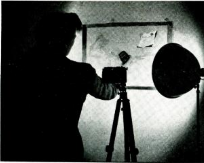
A color slide that shows the route you followed is an important part of your travel record because it helps your viewers to visualize the relationship of the different places. In copying the map, use two lights for even illumination and a meter to help you get correct exposures.
